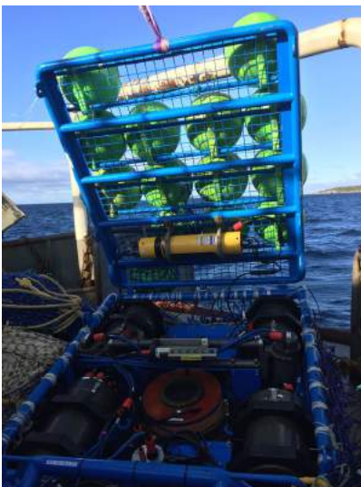
Figure 1-2. Acoustic optical system a, b), attached to the headline of a trawl net with the AOS system, c. attached to the net on Saxon Onwards with the lid open and d. the underneath of the system showing the transducer, camera and light placements for this voyage.
