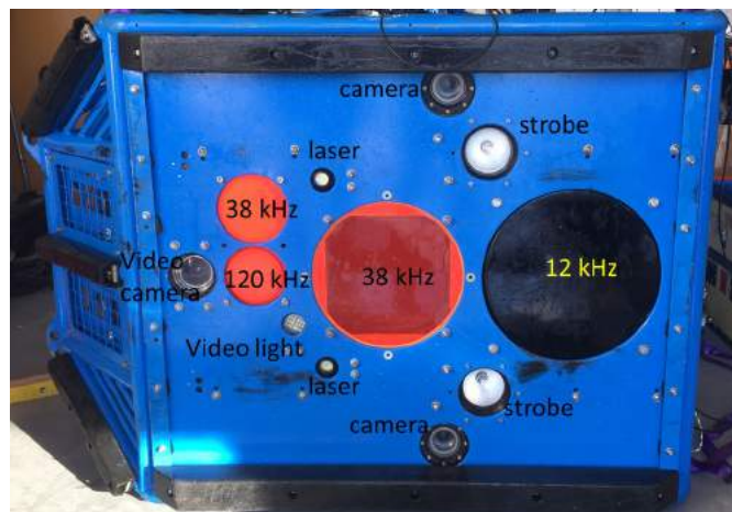
Figure 1-2. Acoustic optical system a, b), attached to the headline of a trawl net with the AOS system, c. attached to the net on Saxon Onwards with the lid open and d. the underneath of the system showing the transducer, camera and light placements for this voyage.
